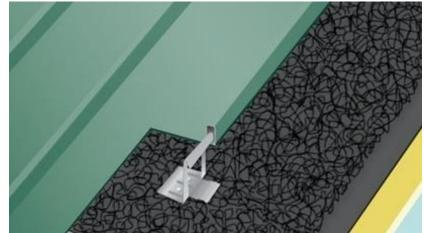
As illustrated here, water vapor moves from the humid interior through the attic and permeable roof materials and through gaps, both in the sheathing and adjacent to the ridge vent. Moisture buildup occurs on the bottom of a colder metal roof surface.
