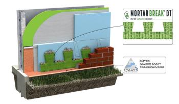
Mortar Break® DT is available in .4", 1" & 2" thicknesses
