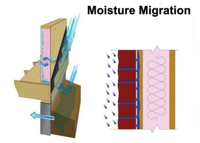
External sources include rain, wind, and snow. Wind-driven rain can be forced into small openings in the exterior cladding at joints, laps, utility cutouts, electrical outlets, nail holes, and more. Trapped moisture can expand through freeze/thaw cycles and damage certain absorptive claddings, such as brick, stone, and stucco.
