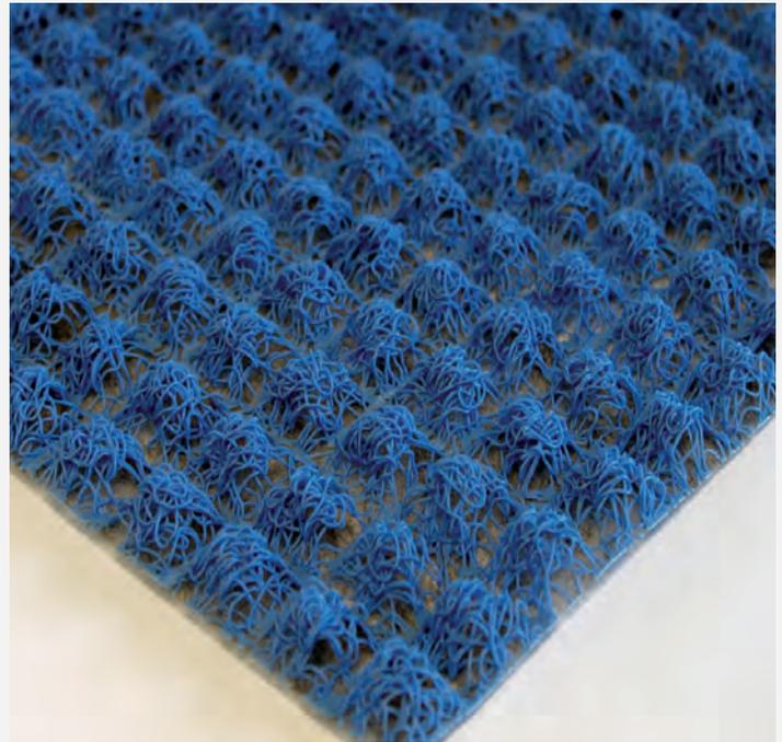
When building exterior walls with stone, stucco, brick, cedar, or fiber cement siding, an effective rainscreen system is imperative. Mortairvent® is a drainage and ventilation system specifically designed for use with most exterior siding materials, primarily in residential and mixed use structures. Mortairvent® is available in 0.125 in. (3mm), 0.25 in. (6mm) or 0.40 in. (10mm) thicknesses.
