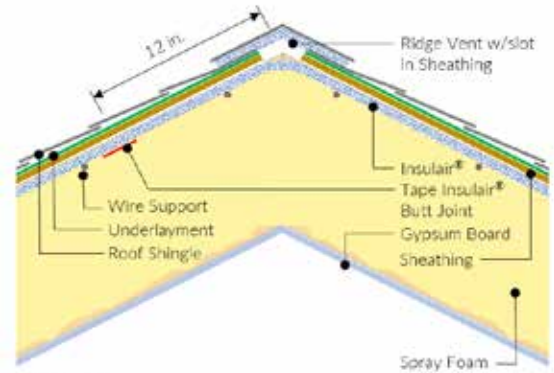
Detail E Ridge Vent/No Ridge Beam
